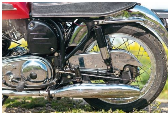
Lashings of Chrome, with an effective 18cm rod-operated rear brake, plus alloy rims and a magneto behind the cylinder.
