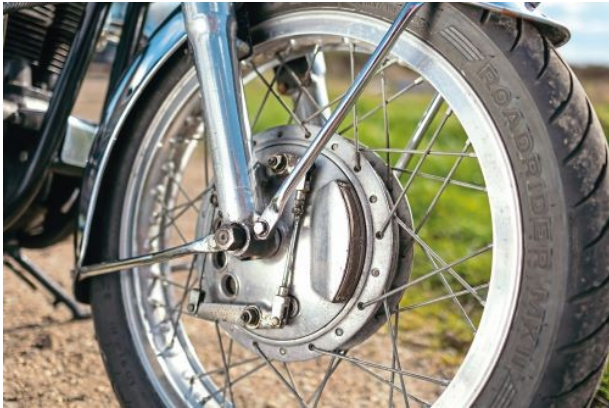
20cm twin leading-shoe front brake from Commando. Not as good as BSA/Triumph equivalent, but this one worked okay.
