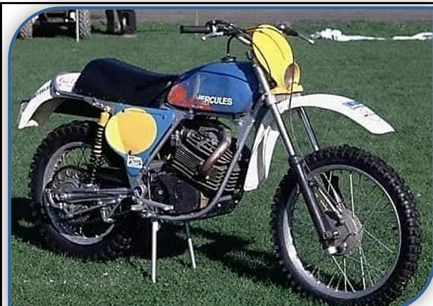
The 1974 Hercules W-2000 used a Sachs-sourced Wankel,
